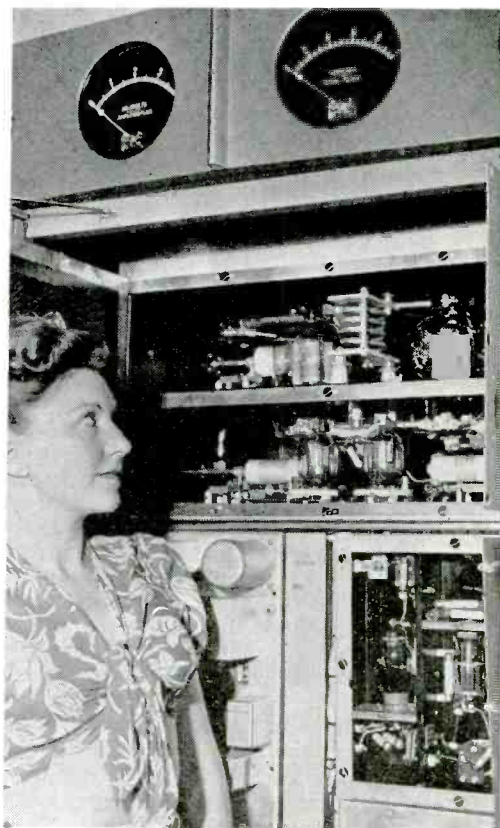
Looking into W.E. 1 kw FM transmitter; final on top shelf; multipliers below
