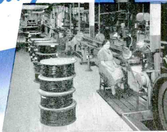
Clean, smooth, properly centered polyethylene covered wire is extruded by this machine.
