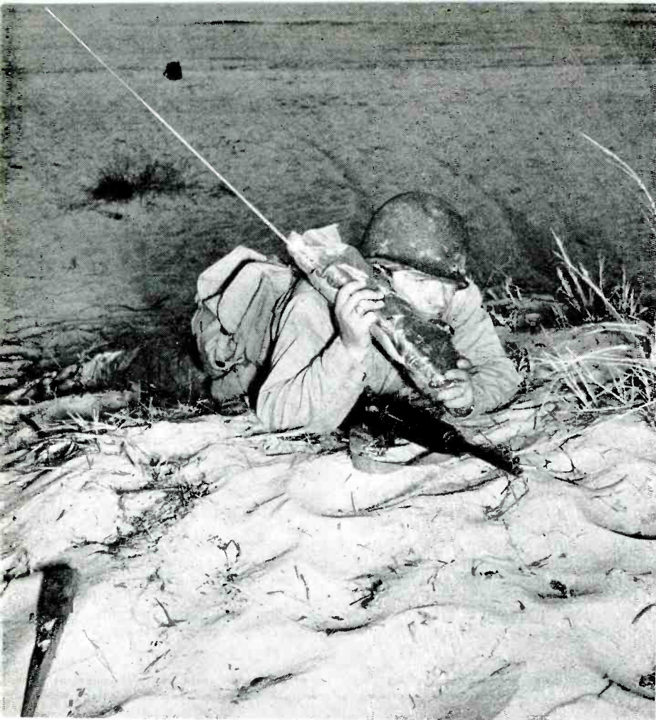
Even the ubiquitous "Handi-Talkie" must be adequately waterproofed, here with a special type of covering put on as an expedient by the soldier himself to permit operation under all conditions
