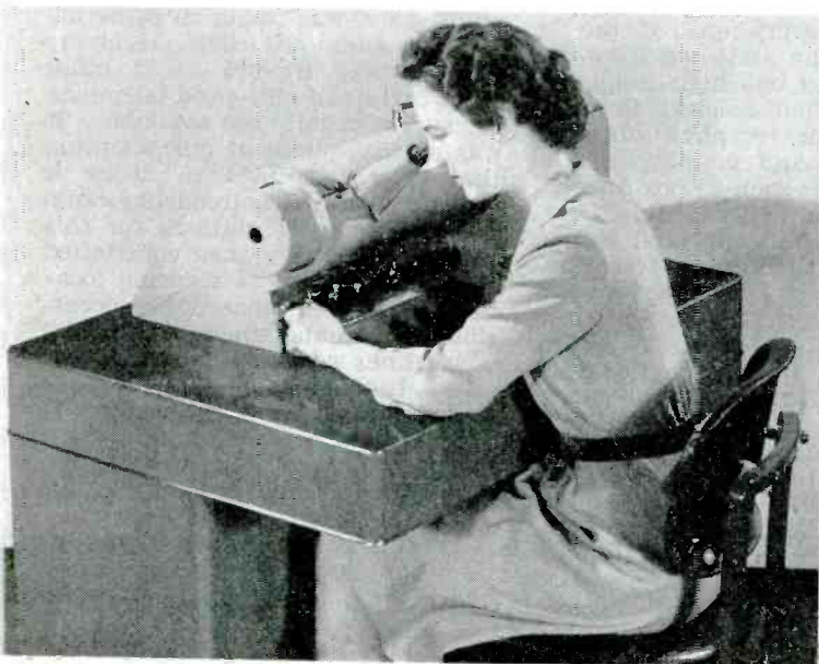
RCA's type EMC electron microscope is a simplified version of the larger model in console form intended primarily for industrial use
