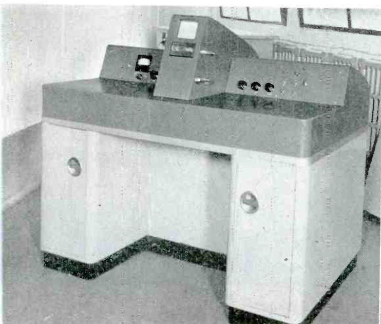
RCA's type EMC electron microscope is a simplified version of the larger model in console form intended primarily for industrial use
